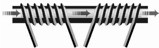
Figure 2. Sensing coil design.
